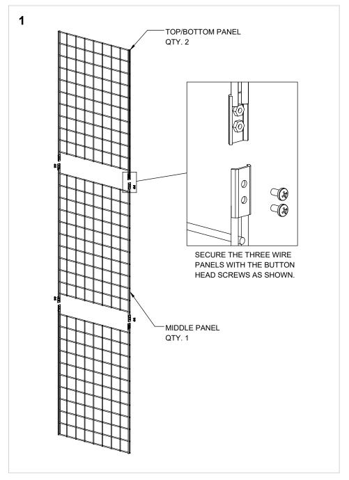
2X8 Portable Grid Panel SHEET 1 OF 1
