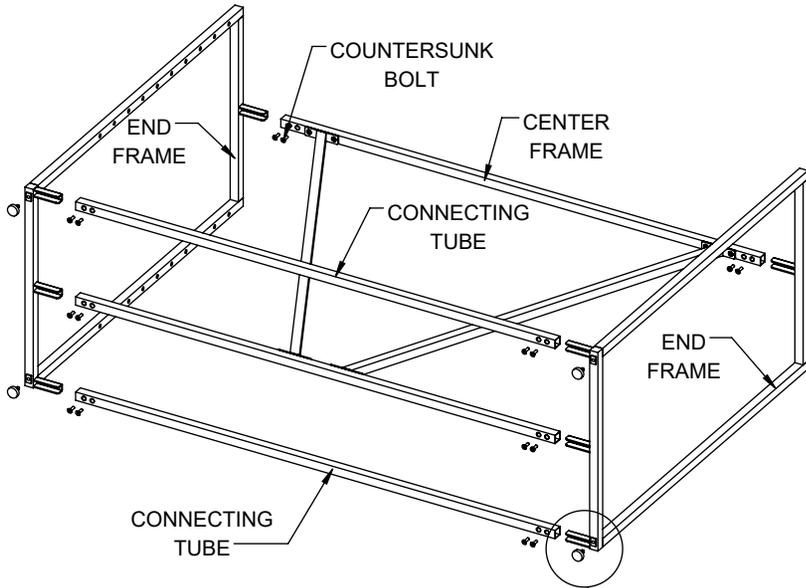
**\*NOTE:** IF THEY ARE NOT ALREADY INSTALLED, THREAD LEVELERS INTO END FRAMES.
